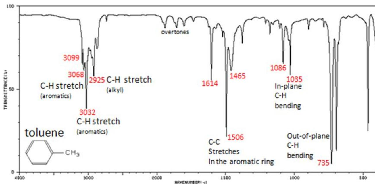
Figure 6. Infrared Spectrum of Toluene
