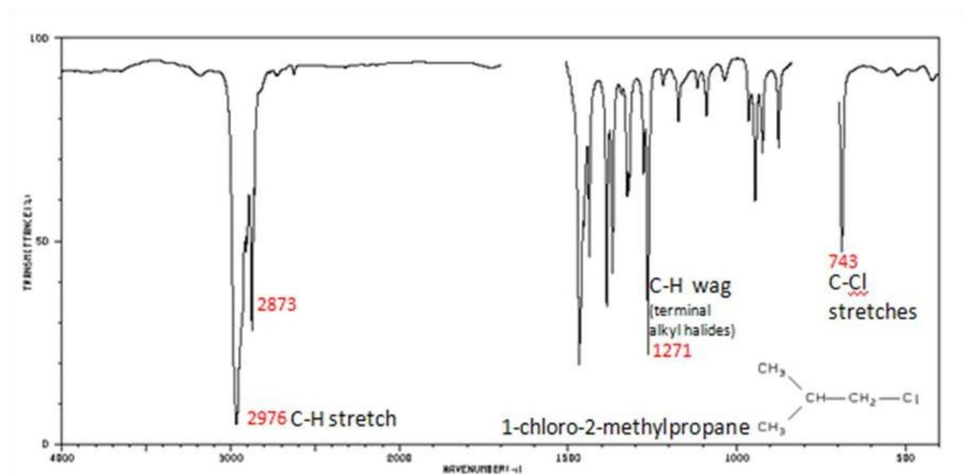
Figure 13. Infrared Spectrum of 1-chloro-2-methylpropane
