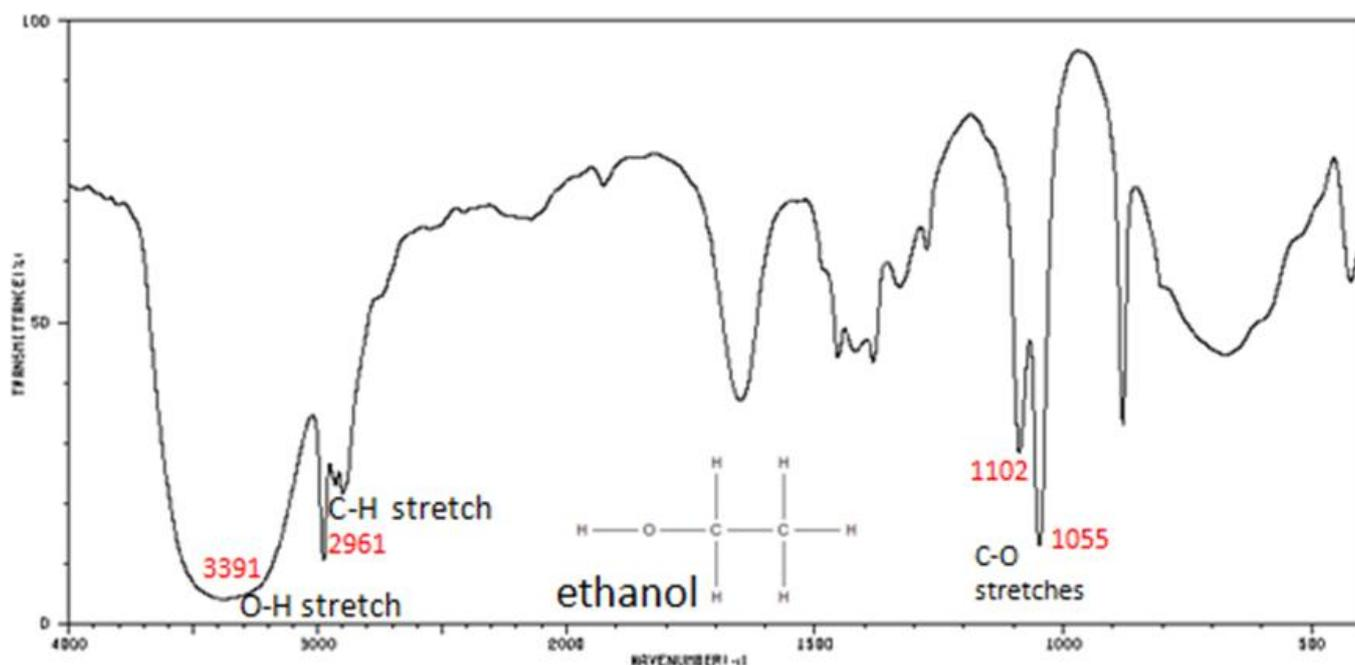
Figure 7. Infrared Spectrum of Ethanol
