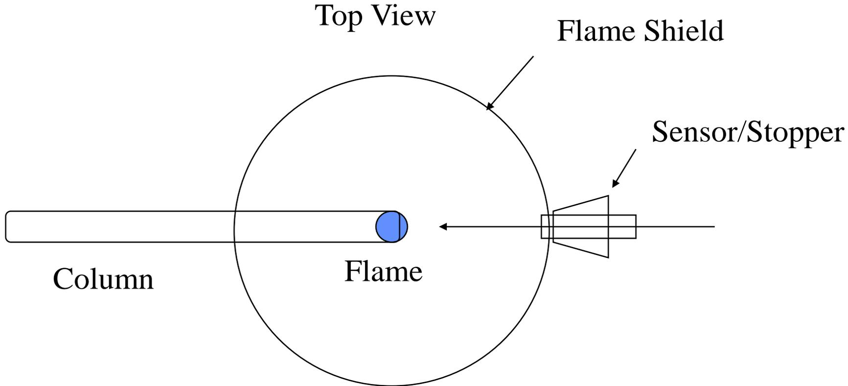
1. Remove sensor from stopper and sight through tube.
