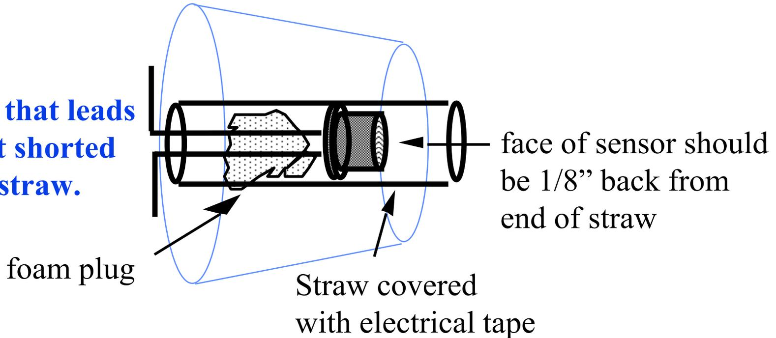
**Note: The sensor should be tested by connecting to computer and checking voltage in light and with sensor face covered with your finger.**
