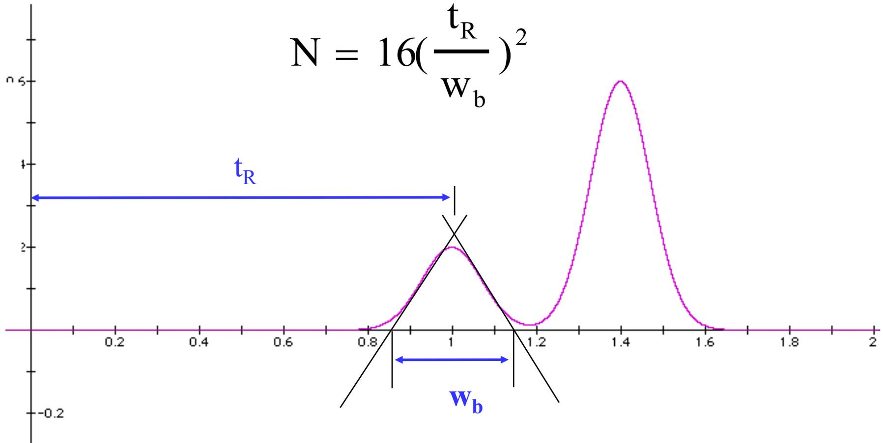
$t_R$  is the retention time; it is measured from the injection peak (or zero) to the intersection of the tangents.
