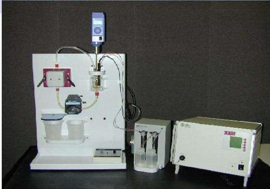
Electroacoustic - **Colloidal Dynamics Acoustosizer** powders/slurries
