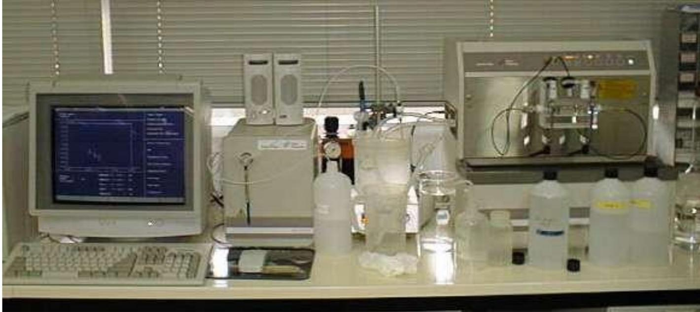
Streaming Potential – **Paar Physica EKA** granular particles, surfaces
