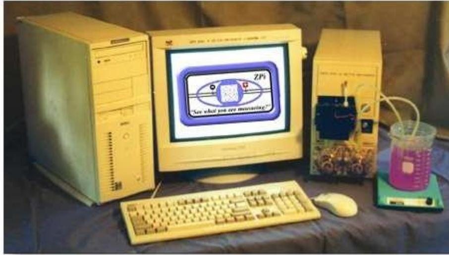
Electrophoresis - **Zeta Mark 21** particles ~ .10 microns- 300  $\mu\text{m}$
