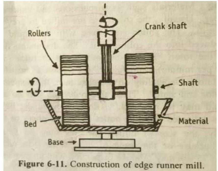
Figure 6-11. Construction of edge runner mill.
