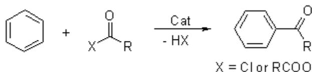
This electrophilic aromatic substitution allows the synthesis of monoacylated products from the reaction between arenes and acyl chlorides or anhydrides. The products are deactivated, and do not undergo a second substitution. Normally, a stoichiometric amount of the Lewis acid catalyst is required, because both the substrate and the product form complexes.
