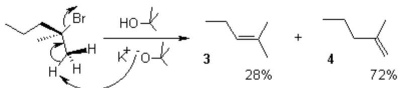
The use of sterically hindered bases raises the activation energy barrier for the pathway to the product predicted by Saytzeff's Rule. Thus, a sterically hindered base will preferentially react with the least hindered protons, and the product distribution will be controlled by kinetics.
