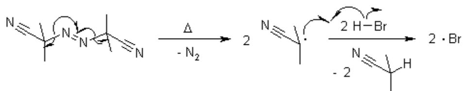
The reversal of the regiochemistry of addition is the result of the reversal of the order in which the two components add to the alkene. Radical addition leads to the formation of the more stable radical, which reacts with HBr to give product and a new bromo radical:
