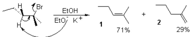
Saytzeff Rule implies that base-induced eliminations ( $E_2$ ) will lead predominantly to the olefin in which the double bond is more highly substituted, i.e. that the product distribution will be controlled by thermodynamics.
