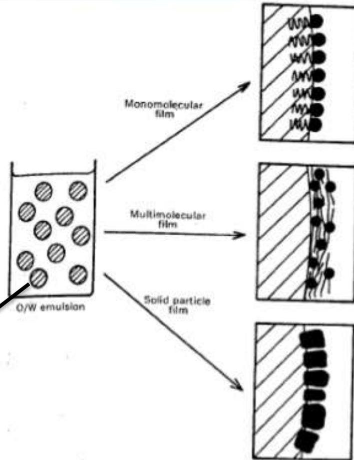
Figure 22-6. Types of films formed by emulsifying agents at the oil-water interface. Orientations are shown for O/W emulsions.  $\bullet$ : oil.  $\square$ : water.
